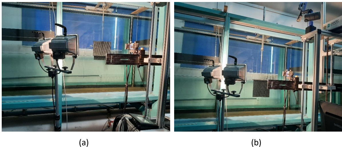
Figure 3- 11. The levelled and installed PIV calibration plate for wind (a) and water (b) velocity field measurements.
