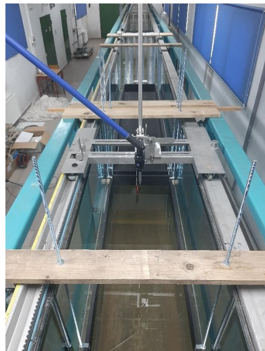
Figure 3- 2. A view of hanged ceiling with the bars (a) and the laser device on top of the plexiglass section of the ceiling (b), showing a view of the wind flume from the top and the top measurement window.
