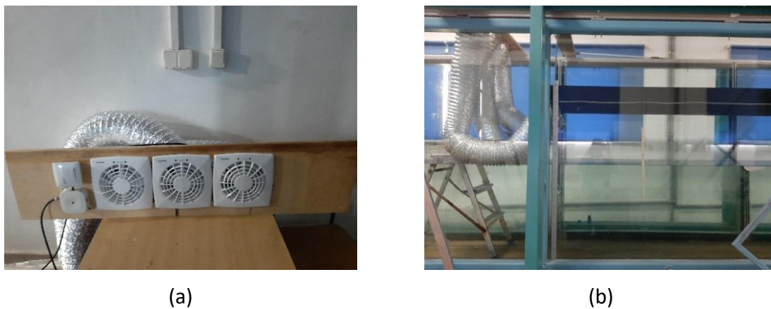
Figure 3- 4. Set up for the wind generator (a), the installation of the wind generators on top of the flume.
